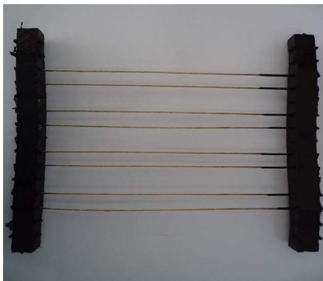
Figure 1. Rubber /steel cord specimen. [Color figure can be viewed in the online issue, which is available at wileyonlinelibrary.com .]
